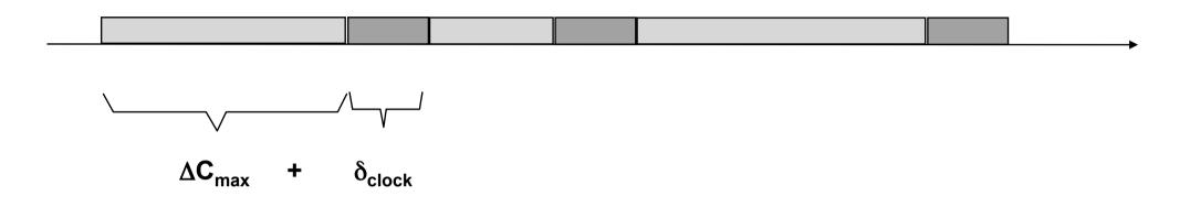
$\Delta C_{max}$  max. time interval (possibly under failure assumptions), which is neccessary to safely transmit a message to the destination
